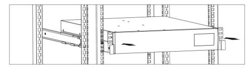
**Step 5:** Fix the UPS in position with 4 screws.
